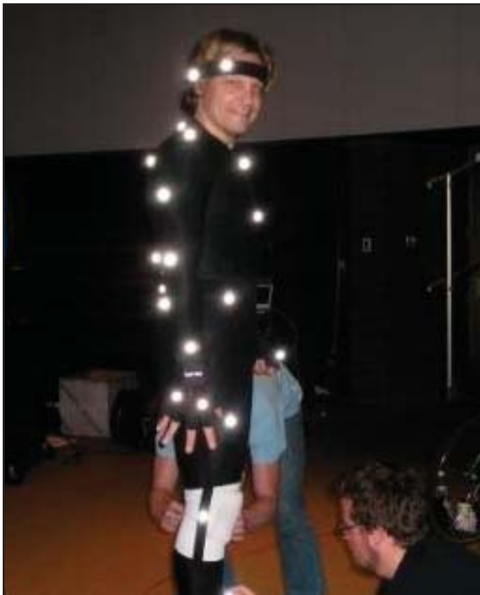
Eddie gets suited up with reflective sensors attached by velcro to a special suit.
